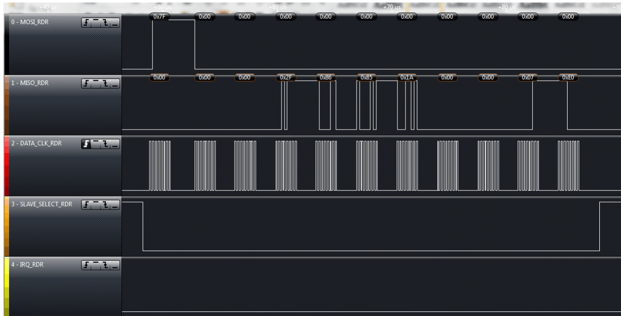
Figure 6-25. Continuous Read of FIFO After Inventory Command
