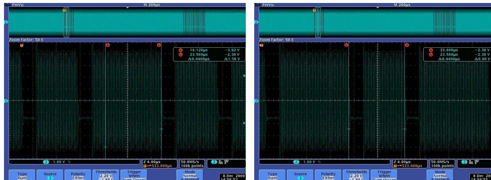
Figure 6-31. Receive Data Bits and Framing Level
